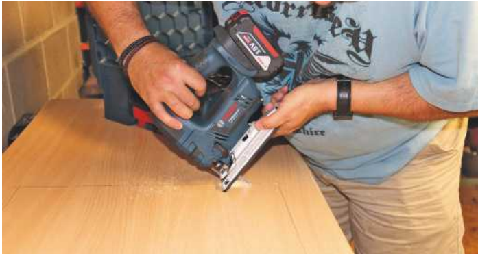
▲ Plunge cuts are easily made with a jigsaw; tilt the saw to start then keep it steady as you begin to tilt it into the work
